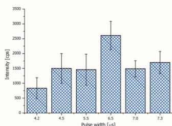
Figure 3: Signal intensities for <sup>103</sup>Rh depending on DOD pulse width ( $f_s=0.54$  kHz)
