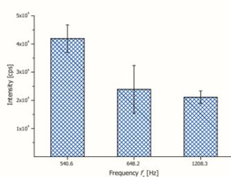
Figure 4: Signal intensities for <sup>103</sup>Rh depending on DOD frequency (pulse width 4.5  $\mu$ s)
