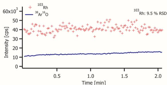
Figure 2: Very first DOD-ICP-MS coupling, signal stability of <sup>103</sup>Rh, 100  $\mu$ g  $L^{-1}$
