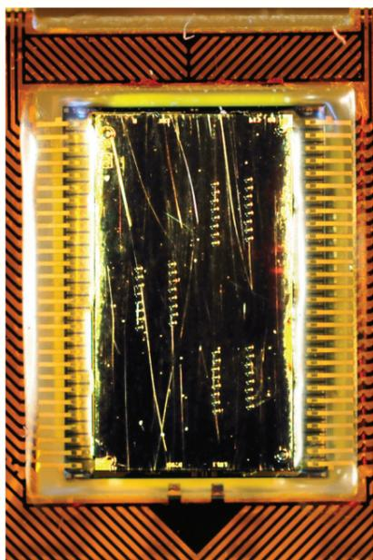
Figure 1: Nozzles of a color cartridge printer head
