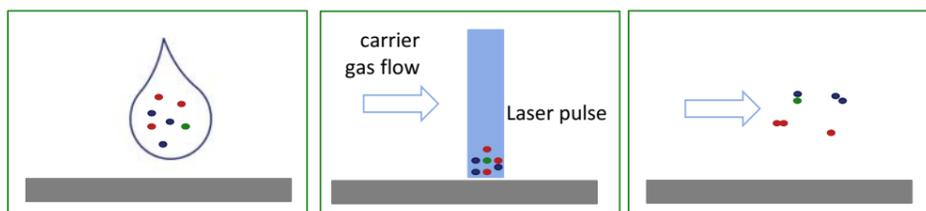
Figure 2: Schematic description of the novel calibration strategy based on laser ablation of dried residues of picoliter droplets from liquid standard solutions.
