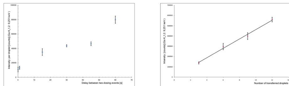
Figure 4: (left) TXRF-signal intensity per dosing event (9 replica) versus the delay between two events; (right) TXRF calibration curve: intensity versus number of transferred droplets (delay time 45 s).
