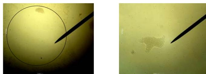
Figure 5: Microscopic images of dried residues dispensed by a microliter pipette (500 nl droplets, transferred mass: 500 pg Se).
