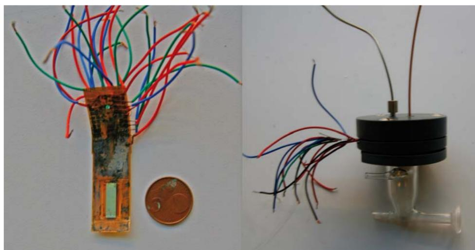
Figure 1: Schematics of a low-dead-volume interface for coupling HPLC with ICP-MS based on a modified HP45 printing cartridge.
