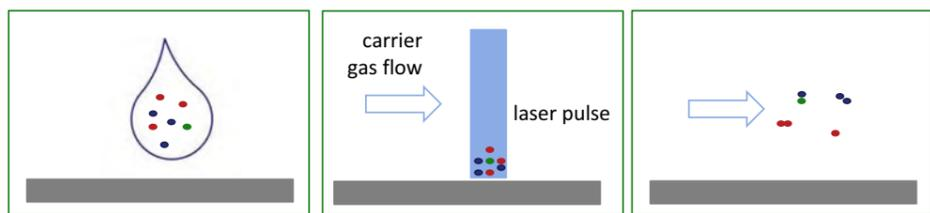
Figure 2: Schematic description of the novel calibration strategy based on laser ablation of dried residues of picoliter droplets from liquid standard solutions.
