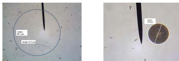
Figure 4: Left: Microscopic images of dried residues. Left: dispensed by a microliter pipette (1  $\mu\text{L}$  droplet, 1 ng Se). Right: dosed by DOD-generator (see above) (5 droplets, delay time 10 s, approx. 1 ng Sr absolute mass).
