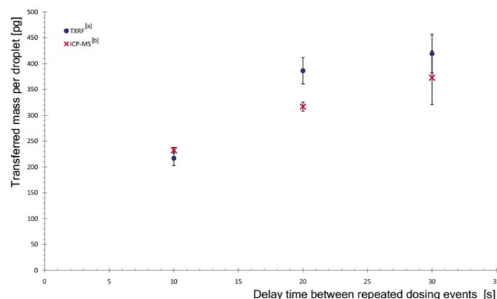
Figure 3: Determined transferred mass (Sr) per droplet (5 replica) versus the delay time between repeated dosing events; [a] 5 droplets per sample (quartz disc); [b] 50 droplets per sample diluted to 1 mL (1  $\mu\text{g/l}$  Rh internal standard).
