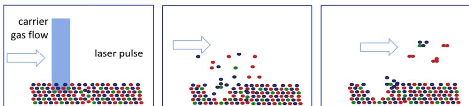
Figure 1: Schematic description of a conventional calibration based on laser ablation of solid standard reference materials.
