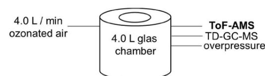
Fig.2: Experimental setup of the seaweed incubation experiments
